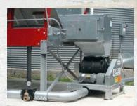
**Remote Control Enclosure** offers mounting flexibility for convenient location of operator controls for the pneumatic conveying system. The weather-resistant enclosure includes control switches, pressure gauge, amp meter, and high-pressure limit switch.
