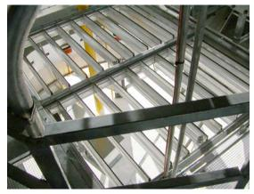
Fresh air along with electrical conduits and gas piping enter at the bottom of the dryer and not through the grain columns. This promotes even grain flow and efficient drying. Air inlet louvers are adjustable to control the volume of cool air entering the dryer.
