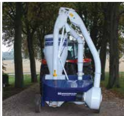
Loading equipment hydraulically folded for the transport position.
