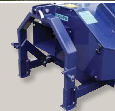
Three-point attachment to tractor lift.
