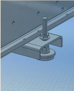
When GUARDIAN® Series Centrifugal Fans require a foot-mount, Brock's high-strength, adjustable foot structure with dampening pad assists with leveling the unit and provides the fan support needed for smooth operation.
