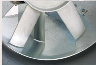
**Air vanes** are a standard feature on all 18-inch (457-mm) diameter and larger fans. The vanes aid efficient airflow at higher static pressures by reducing air turbulence.
