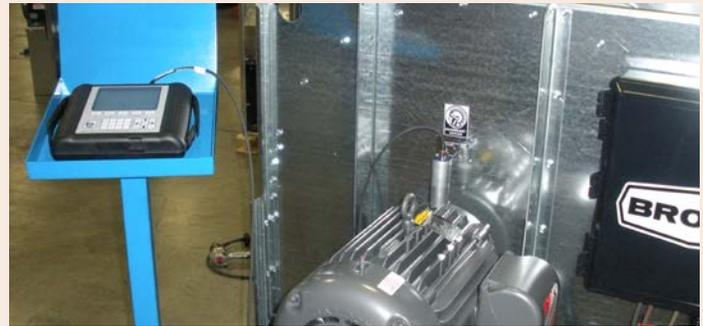
As a part of Brock's high standard of quality and reliability, all GUARDIAN® Series Centrifugal Fans are factory-tested for fan balance to minimize performance-robbing vibration.
