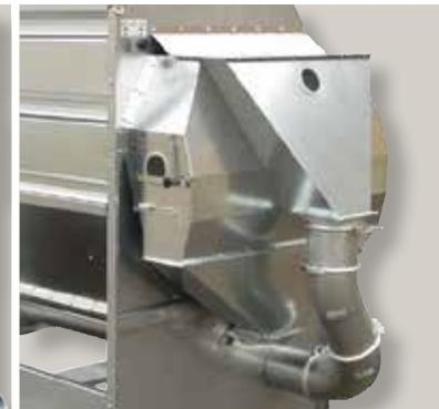
A handle placed on the outside cabinet makes it easy to adjust the aspirator function without any tools.
