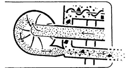
Impurities separated by screens and aspirator discharged into the trash blow line. Impurities separated by screens and aspirator discharged separately.
